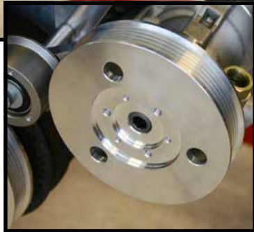
Photo 13: Press power steering pulley (619-A) on with an install tool or bolt and washer as shown. When properly installed pulley should be flush with top of shaft as shown.
