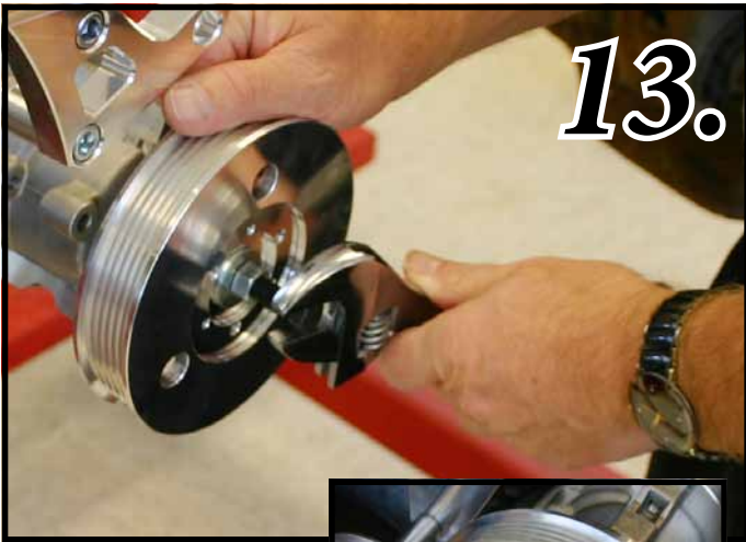
Photo 13: Press power steering pulley (619-A) on with an install tool or bolt and washer as shown. When properly installed pulley should be flush with top of shaft as shown.
