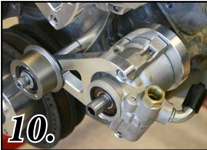
Photo 10: Once the power steering bracket has been installed to the block there is enough room behind the bracket to secure the Remote Power Steering Pump (P320) to the bracket using two 8mm x 1.25 x 25 mm (S551) socket head caps screws installing from the back. Install Idler Bracket (20068-A) with two 8mmx25 mm SHCS (S551) to the front of the power steering pump.
