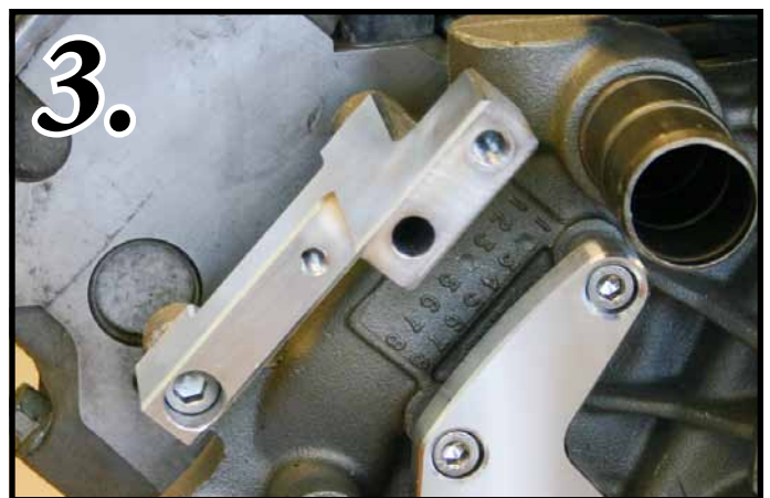
Photo 3: Install Rear A/C Bracket (20067-B) to the water pump as shown using one 10mm x 30mm SHCS (S561) bolt in the lower mounting hole. Snug only at this time.
