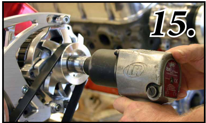
Photo 15: Install Alternator Fan (221) and Alternator Pulley (208-A) and tighten alternator pulley nut (impact to 90 ft, pounds). Check and tighten all bracket bolts and alternator and A/C lower mounting bolts, turn engine over once by hand to check for any belt rubbing and proper belt alignment. Run engine three minutes and check belt tension again.
