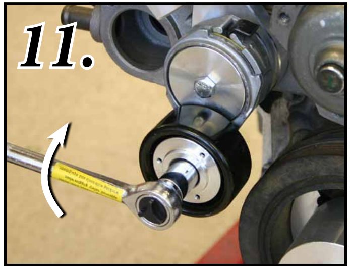
Photo 11: Temporarily mount the OEM style tensioner (P756) to Tensioner Base (20069-A) using one 3/8"-16 x 2 1/4" Hex Head Bolt (S324) , Be sure to align pin on rear of tensioner with hole in tensioner base. This will aid you in removing the tensioner pulley. Remove the pulley bolt using a 15mm wrench and discard the washer.
