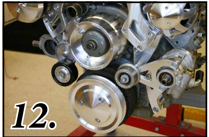
Photo 9: Apply Loc-Tite to the threads of the three 3/8"-16 x 1" SHCS (S248) and install Crank Pulley to the March Crank Adapter Hub
