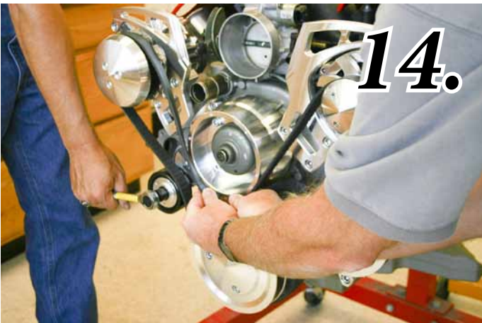
Photo 14: Have an assistant pull back on the spring loaded tensioner and rap the belt around the system pulling the belt over the bottom of the water pump last as shown.
