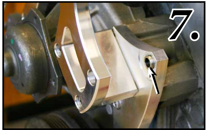
Photo 7: Install threaded bushing (453) in Rear Alternator Support Bracket (20066-B) as shown.
